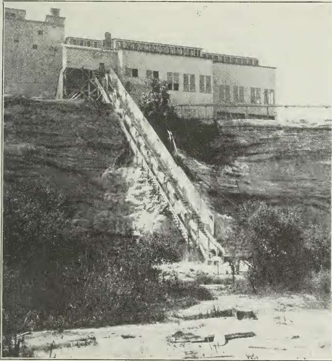
Fig. 26. Drag-belt elevator. (Photograph by courtesy of Ottawa Silica Company.)
